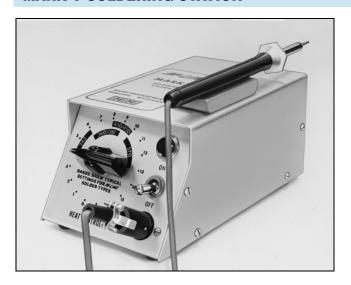
A time-proven precision soldering instrument for miniature and/or delicate soldering applications. Full 25-watt rating in 17 selector positions to handle all M-LINE solder alloys except 1240-FPA. Magnetic solder pencil holder and flexible, burn-resistant cord. Lightweight soldering pencil (1.1 oz [31g]). Specify 115 or 220Vac, 50 or 60Hz operation.
